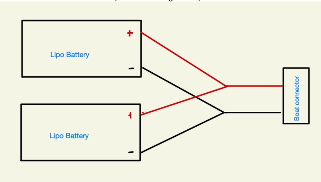
Figure B-2: Battery connection [13]
